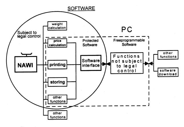
Figure 2: Example of a software structure of a PC-based weighing system
