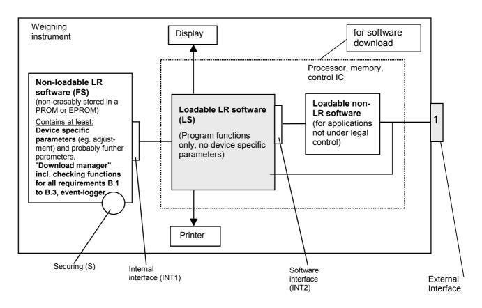
Figure 4: Software download into a weighing instrument with separation of the LR software from the non-LR software by a protective software interface (INT2) (see requirement B.5).
